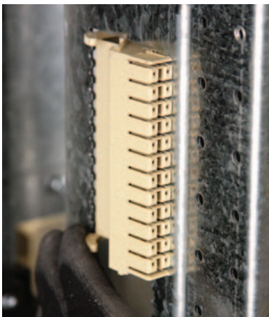
FIGURE 32. Uninstall the Control Terminal Block
