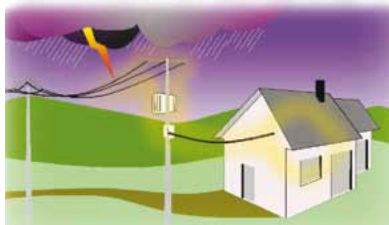
Direct lightning strike on an overhead line
