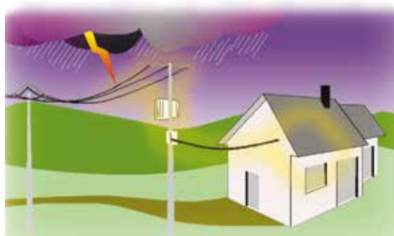
Direct lightning strike on an overhead line
