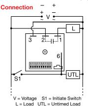
The untimed load is optional. S1 is not used for some functions. Dashed lines are internal connections.
