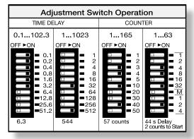
One or more switches must be ON for proper operation.
