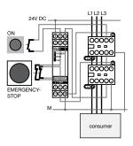
Internal standard circuit diagram of safety relay C 6701 with solid-state output.
